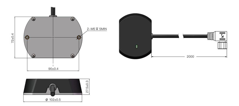
Figure 2.9 Connection Box - Connection (Unit: mm)
