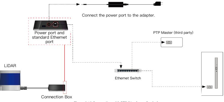
Figure 2.13 Connection with PTP (Hardware Device)
