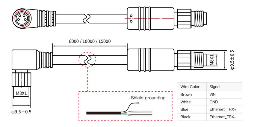
Figure 2.8 Extension Cable and Connector Size
