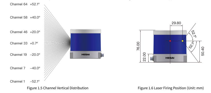
The vertical resolution is unevenly distributed across all channels, as illustrated in Figure 1.5 and detailed in Appendix I (Channel Distribution).
