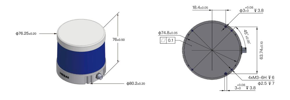
Figure 2.1 Isometric View (Unit: mm)
