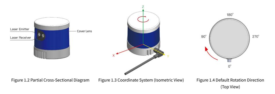
Laser emitters and receivers are attached to a motor that rotates horizontally.
