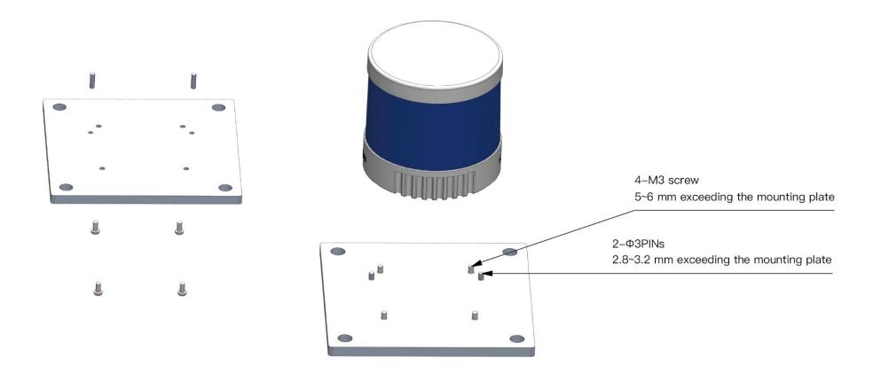
Figure 2.3 Recommended Installation
