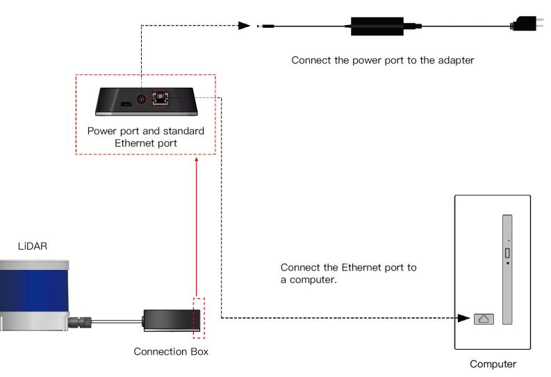
Figure 2.12 Connection with PTP (Software Device)
