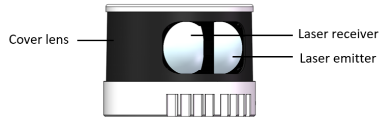
Figure 1. Partial cross-sectional diagram
